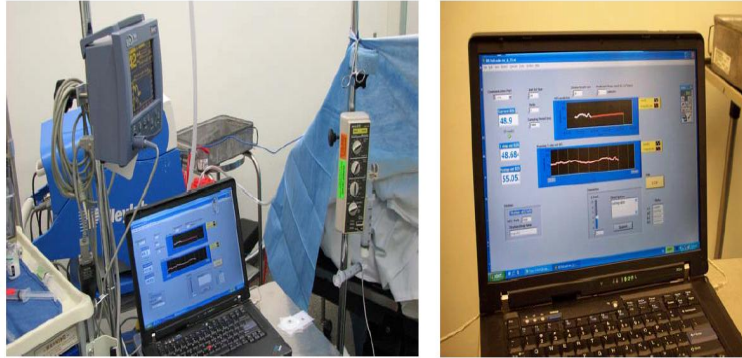
Figure 28: BIS prediction system hardware setup
